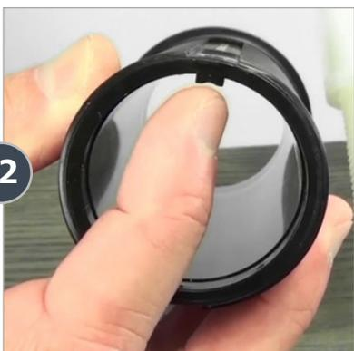
Align the groove in the white stem with the tooth inside the lower portion of the black sleeve. Sliding the stem down in, as far as possible.
