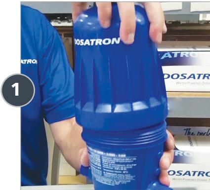
Begin by removing the piston from your Dosatron injector. Unscrew and remove the bell housing (you may use a universal strap wrench), pulling the piston out of the body. Set the bell housing and body aside.
