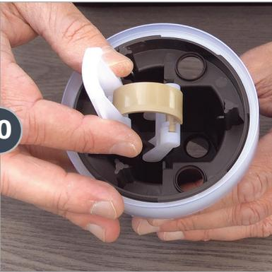
To demonstrate the alignment of the push rod assembly, the curved top would face inward, inserting the push rod into the single hole. This is where the connecting rod sits in the piston.
