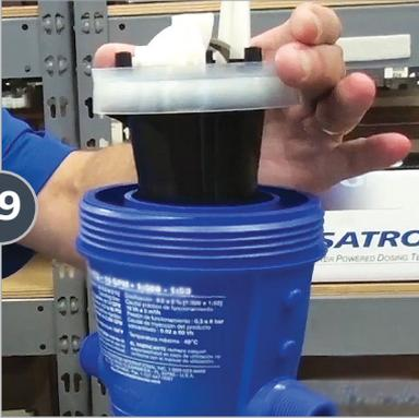
Carefully press the piston back into the injector and install the bell housing.
