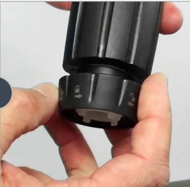
Unscrew and remove the lock nut.
