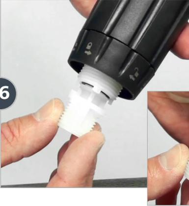
Install the new **Check Valve Assembly** (Part #: **PJDI234**) into the stem. Make sure it is in the position shown before inserting into the stem.
