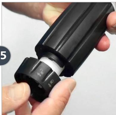
Thread on the lock nut and hand tighten.
