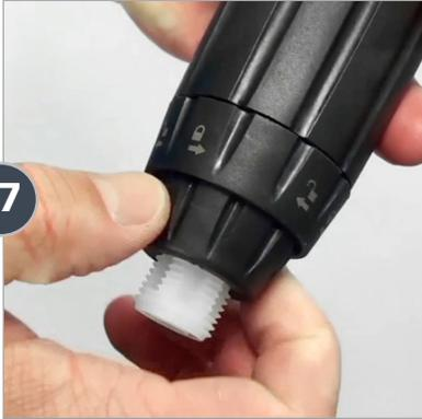
Reinstall the check valve nut.
