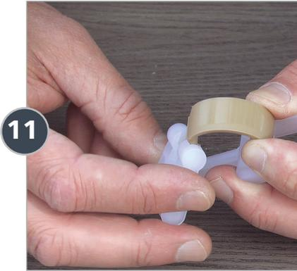
Slide the other end of the Omega spring into the new **Connecting Rod** (Part #: **PDI649**). The key to this step is to make sure the curved top of the push rod faces in the same direction as the Omega spring.
