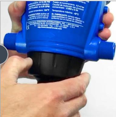
Unscrew the injection stem nut.
