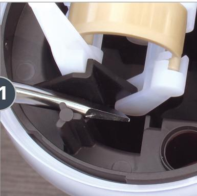
The key is to make sure the white connecting rod drops into the notches inside the piston shell.
