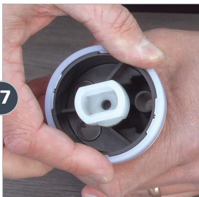
Install the new **Lower Flange** (Part #: **PDI644**) the same way.
