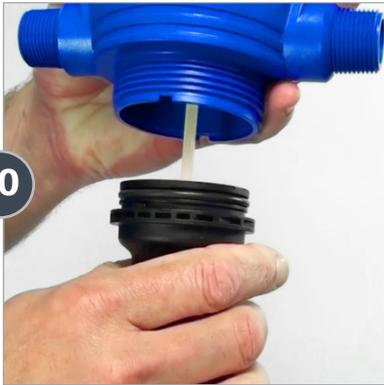
To finish up, carefully insert the plunger into injection stem assembly.
