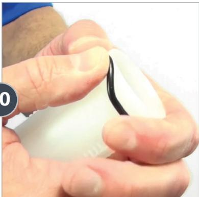
Remove and replace the **Injection Stem O-Ring** (Part #: **JDI120**).
