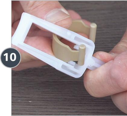
Twist to remove the Omega spring out of the push rod.
