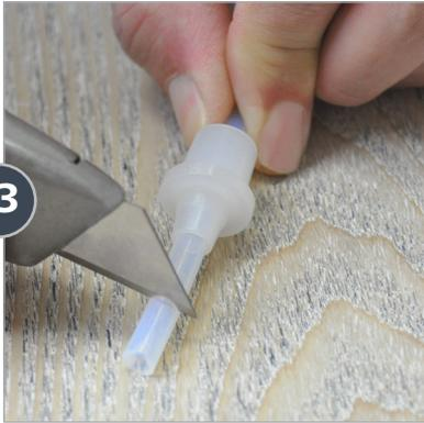
Before installing the suction hose, slide the ferrule back onto the hose. Cut a half inch off the top of the hose.
