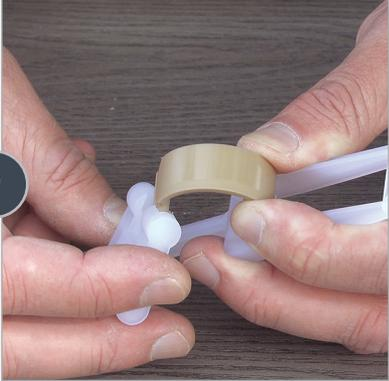
In order to disassemble the push rod, remove the connecting rod off the Omega spring.
