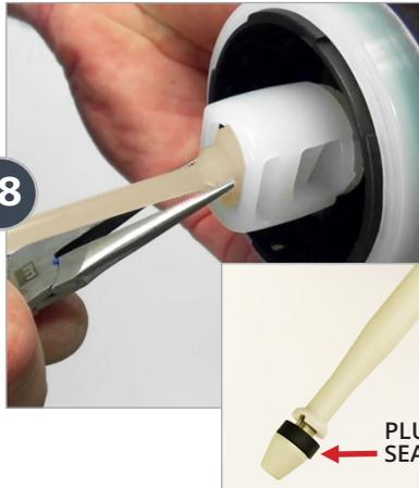
Remove and replace the **Plunger Seal** (Part: **JDI208**).
