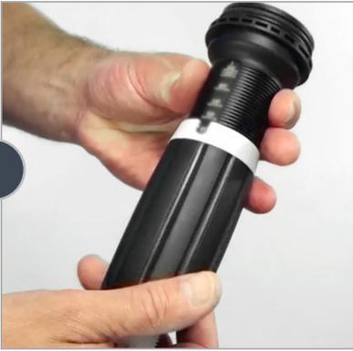
Unscrew and remove the adjusting nut.
