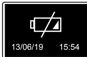
The “low battery” alarm indicates that the remaining battery life is less than 1 hour, and that the battery should be replaced. See MAINTENANCE
