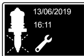
If this alarm appears, you should check the strainer, the general condition of the suction tube and the correct position of the level detection pipe in relation to the strainer or the plunger seal. Recommendation: Perform a diagnosis using the measuring cylinder (see the DIAGNOSIS FEATURES section).
