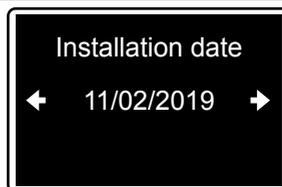
Press to access the total meter values, as well as information concerning the running time, the total volume of water that has passed through the pump (treated and untreated water), and the total volume of treatment (estimated total volume) injected since the installation.
