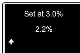
The red LED remains on, and the dosing value flashes until the selected value is reached. (if the expected value cannot be reached, index the dosage as described in the DOSAGE INDEXING section).
