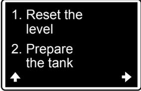
During a vaccination, once you have filled the stock solution tank, the system will prompt you to prime the drinking pipes until the blue dye mixed with the vaccine solution reaches the drinkers. The system will then account for the amount used to prime the system.
