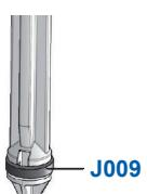
**!** Using tools could damage the plunger and affect the injection rate
