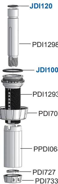
Reinstall "C" clamp by sliding it gently over the thread at the bottom of the white stem. Rotate clamp until it clicks into place.
