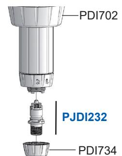
Screw check valve nut (PDI734) back on.
