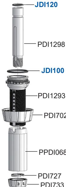
**!** To remove o-ring easily without tools, squeeze it on either side to raise the seal, then slide it over the groove
