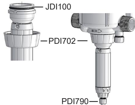
Cut 1" from the tip of the hose in a straight line and insert the hose back onto the bottom of the check valve barb. Screw hose nut (PDI790) back on.
