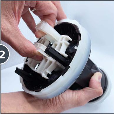
Now, test the piston assembly by carefully pulling the push rod up until you hear a click, then snap the last 3 Valves back on.
