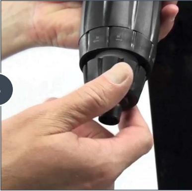
Unscrew and remove the check valve nut.
