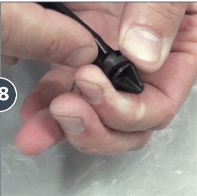
Set the stem aside and pick up the blue body. Remove the Plunger Seal by pinching and rolling it off the plunger.
