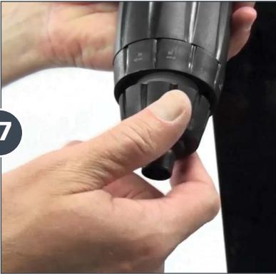
Reinstall the check valve nut.
