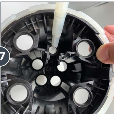
Insert the push rod assembly inside the smaller hole with the top curved portion facing outward (following the curve of the piston).
