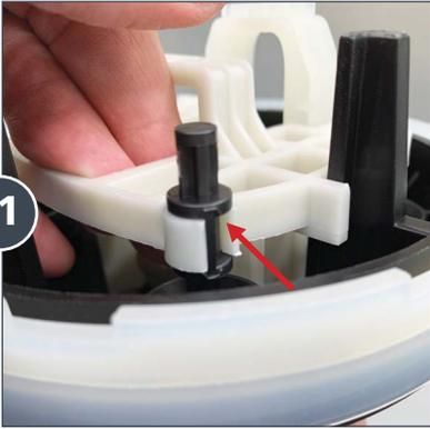
Snap one of the upper valves into the valve guide.
