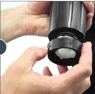
Unscrew and remove the lock nut.
