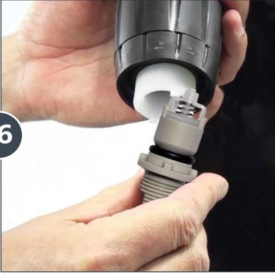
Install the new **Check Valve Assembly (Part #: PJD1232)** into the stem.
