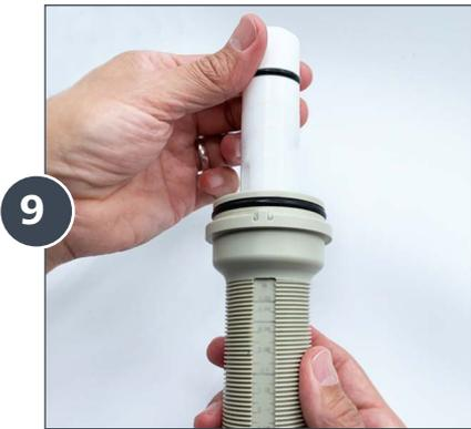
Push the white injection stem up and out of the injection sleeve.
