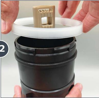
Pick up the **NEW Lower Flange (PDI1092)** and slide it onto the piston shell, with the **V** shape opening facing downward and flat edge facing up. Push down until it sits on the edge of the black piston shell.
