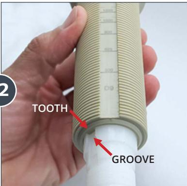
Align the groove in the white stem with the tooth inside the lower portion of the injection sleeve. Slide the stem down as far as possible.
