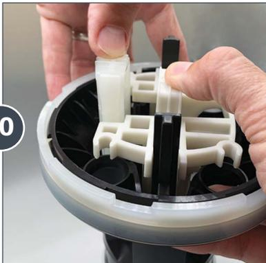
Carefully begin pressing the mechanism (both assemblies) into place inside the piston shell and double check the alignment of both sections.
