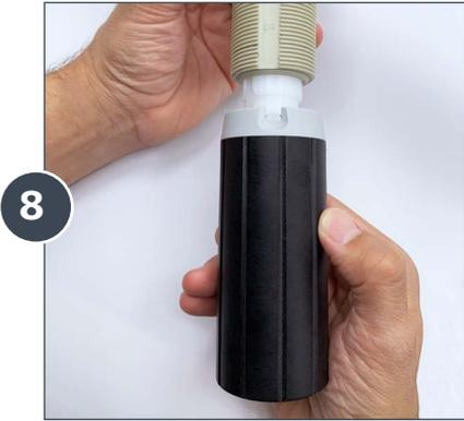
Unscrew and remove the adjusting nut.
